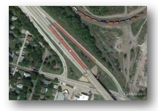
Approximately half of the crashes at this location are vehicles that have struck the median barrier, while the other half are rear-end or side-swipe crashes most likely involving on-ramp traffic preparing to merge with westbound I-70 through traffic. The inside shoulder after crossing the viaduct continues to be narrow through this area which may have contributed to the fixed object crashes with the median barrier.
