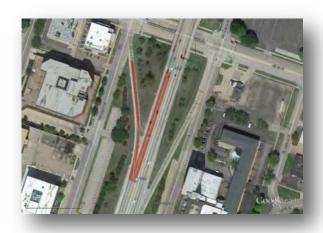
Vehicles enter from 4<sup>th</sup> Street into an added lane on eastbound I-70. There is a short distance between the on-ramp from 4<sup>th</sup> Street and the offramp to 8<sup>th</sup> Avenue. Crashes at this location may be due to vehicles on eastbound I-70 changing lanes and decelerating to exit at 8<sup>th</sup> Avenue in the same lane where traffic from 4<sup>th</sup> Street is accelerating to travel east on I-70.
