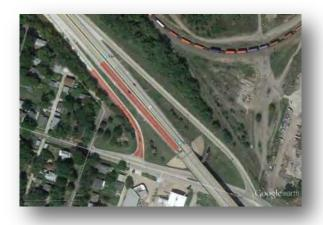
Crashes at this location may be due to the stop-controlled intersection at the ramp terminal causing unexpected queuing along the ramp or to the narrow inside shoulder on mainline eastbound I-70. During the study phase, it was determined that daily traffic queuing occurs during the AM Peak which backs up traffic along mainline eastbound I-70.
