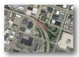
The on-ramp has a very short acceleration lane and there is some difficulty seeing on-coming traffic around the curve to merge. There are also cases where drivers may assume the vehicle ahead of them will accelerate onto mainline, only to have the leading vehicle stop because of the short acceleration lane, leading to a rear-end collision.
